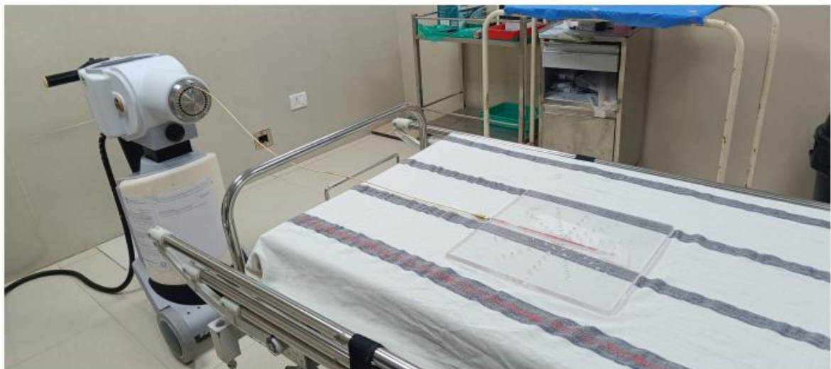
(Fig5: Measurement Setup for In Phantom Dosimetry of Brachytherapy Source)
